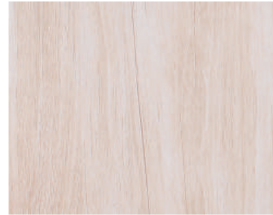
Crack Wood SF 7116
